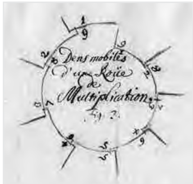
Figure 1 Gottfried Wilhelm Leibniz's drawing of a pinwheel calculator. The caption of the figure reads in French: Movable Teeth of a Multiplication Wheel.
